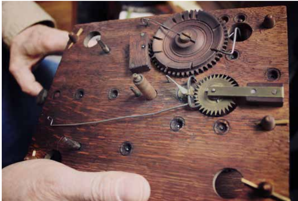
A wooden clock mass—produced in the Connecticut River Valley in the 1820s. "The British wouldn't sell us brass, because they knew we'd turn it into cannon and point it at them," Arnold says.
